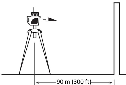
5. Raise/lower the receiver until you get an on-grade reading for the – ▲ axis. Using the on-grade marking notch as a reference, make a mark on the wall.
