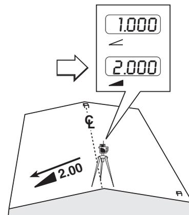
9. Select the axis (↙ or ↘) that you are aligning using the up ⬆ or down ⬇ buttons.
