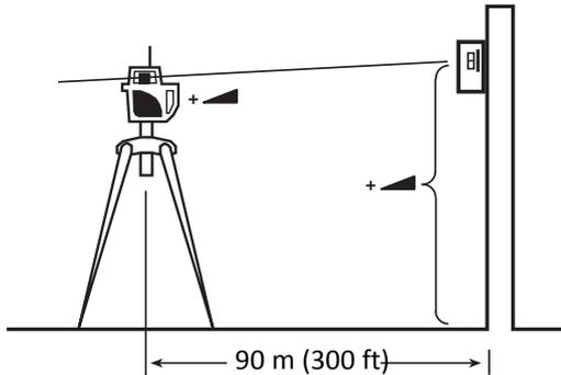
**Note** – For increased precision, use the fine-sensitivity setting (1/16 in / 1.5 mm) on the receiver.
