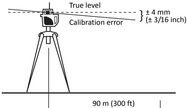
To check the horizontal calibration, you need a tripod with a  $\frac{1}{8}$ -11 threaded mount and a hand-held receiver. If you need to adjust the calibration, having another person to help saves time.
