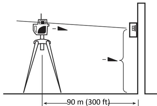
6. Measure the difference between the two marks. If they differ more than 5/16 in. (8 mm), you must calibrate the laser.
