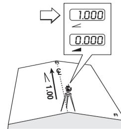
4. Enter the grade value for the side of the road to be graded first into the axis that is perpendicular to the centerline of the road ( $\blacktriangle$ ).
