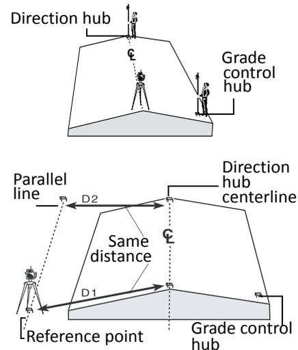
3. Enter the grade value for the axis that aligns with the centerline of the road ( $\blacktriangleleft$ ).
