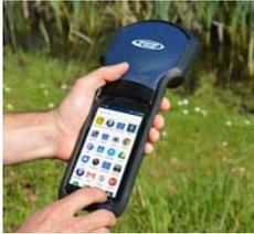
The Spectra Precision SP20 handheld GNSS receiver combines innovative, camera-enabled data collection workflow with a high level of performance in an ergonomic, scalable solution from meter to centimeter accuracy. Rugged and lightweight, the SP20 is easy to use and highly accurate. It is the optimal tool not only for cadastral, construction or topo surveys, but also for a range of GIS projects, including data collection, inspection and maintenance.
