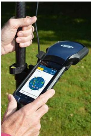
Insert the SP20 into the bracket so that it is pinched where you would normally hold it in your hand. That way you keep the rear camera clear and preserve access to the Power button.
