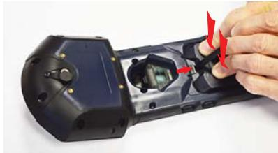
3. Insert the tip of the battery door opener into the recess (top-left corner of the battery door, see also *page 3*) and gently push the opener to release the door out of the unit.
