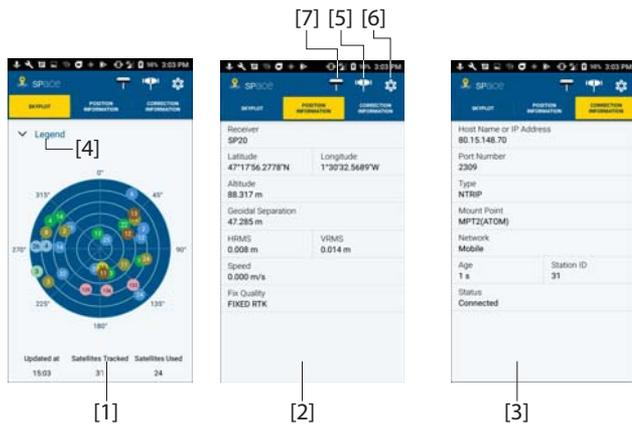
The SKYPLOT tab ([1]) is a polar diagram showing the location in the sky of each tracked satellite.
