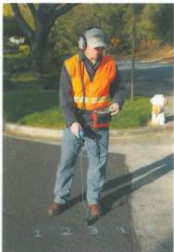
Adjust the sensitivity, change the filters, and use the Noise Reduction, if needed. Do you hear the leak?
